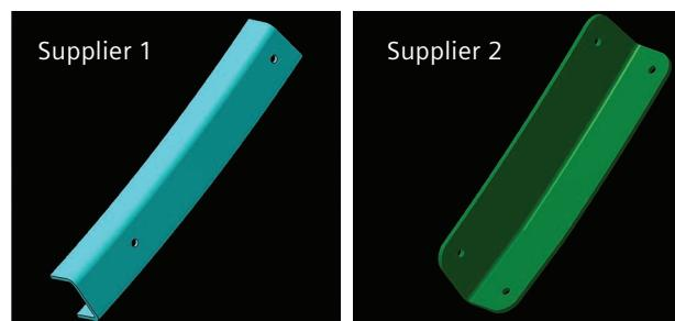
*Syncrofit provides clear and concise information on the initial fabrication state for airframe components by generating condition of supply models.*
